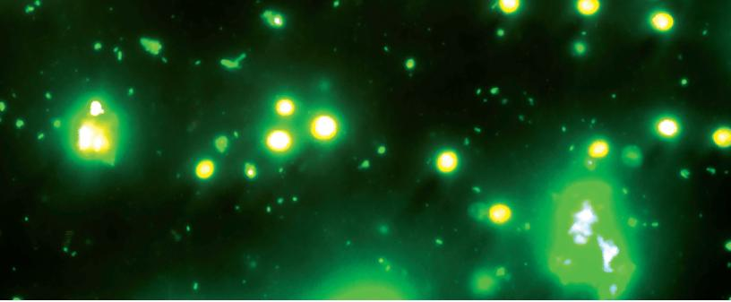
SEEING SPOTS: Some ethanol plants use fluorescence microscopes to detect bacterial infections and maintain yeast health. The microscopes allow technicians to see a mosaic of greens and reds that indicate the type and amount of cells in a sample.
